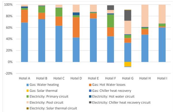
Fig. 10. Hot water production and distribution primary energy disaggregation
