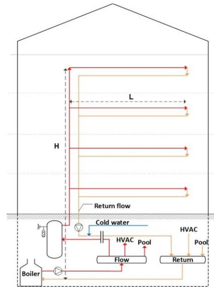
Fig.2. Hot water supply and distribution system
