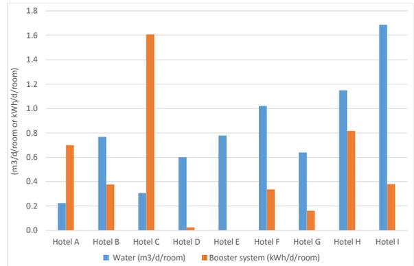
Fig. 8. Booster pumps average daily water and energy consumption
