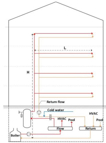
Fig.2. Hot water supply and distribution system
