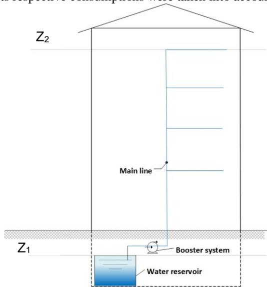
Fig. 1. Cold water supply system with reservoir and booster
